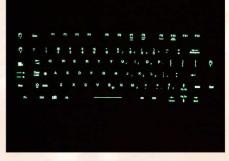
NVIS BACKLIT KEYS
