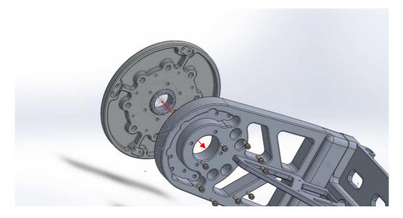
Center the plate with the insert ring and turn the adaptor plate, until your screws hit the threads. Use the torque recommended by your screw manufacturer
