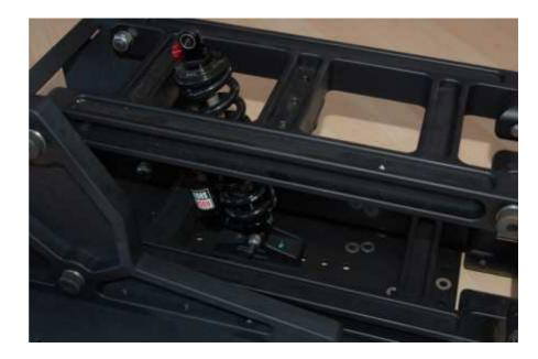
Turn damper to loosen lower thread
