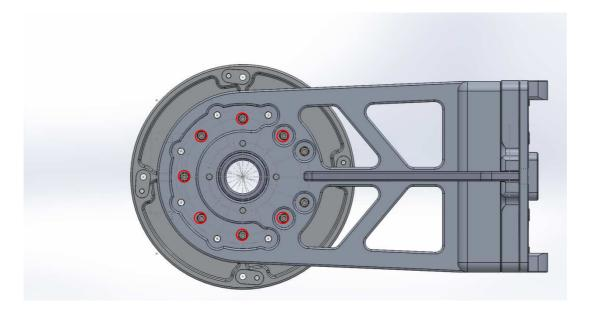
Use the seven marked holes for M5  $\times$  16 philips head screws and 5  $\times$  10 washer all stainless steel
